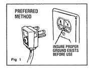
three-prong (grounding) wall outlet (Fig. 1) to minimize the possibility of electric shock hazard from this appliance.
